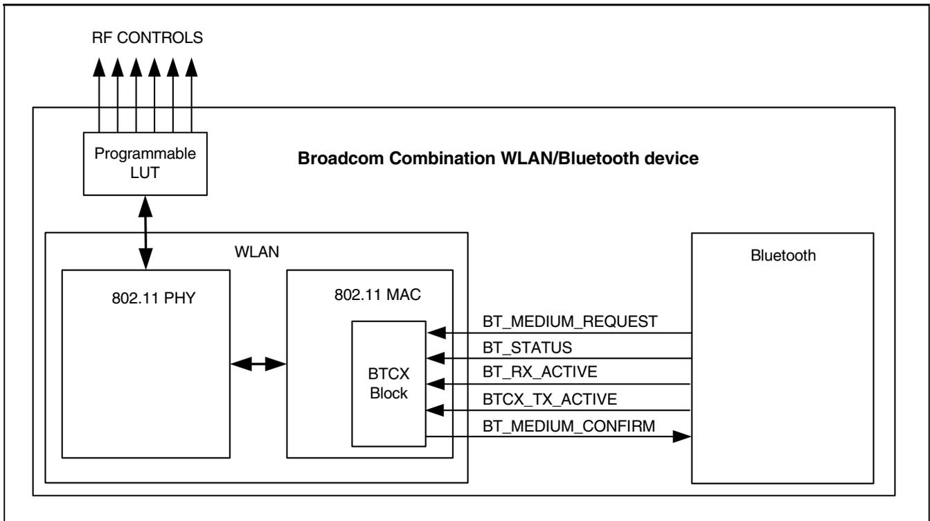
Figure 2: Packet Traffic Arbitration Architecture
