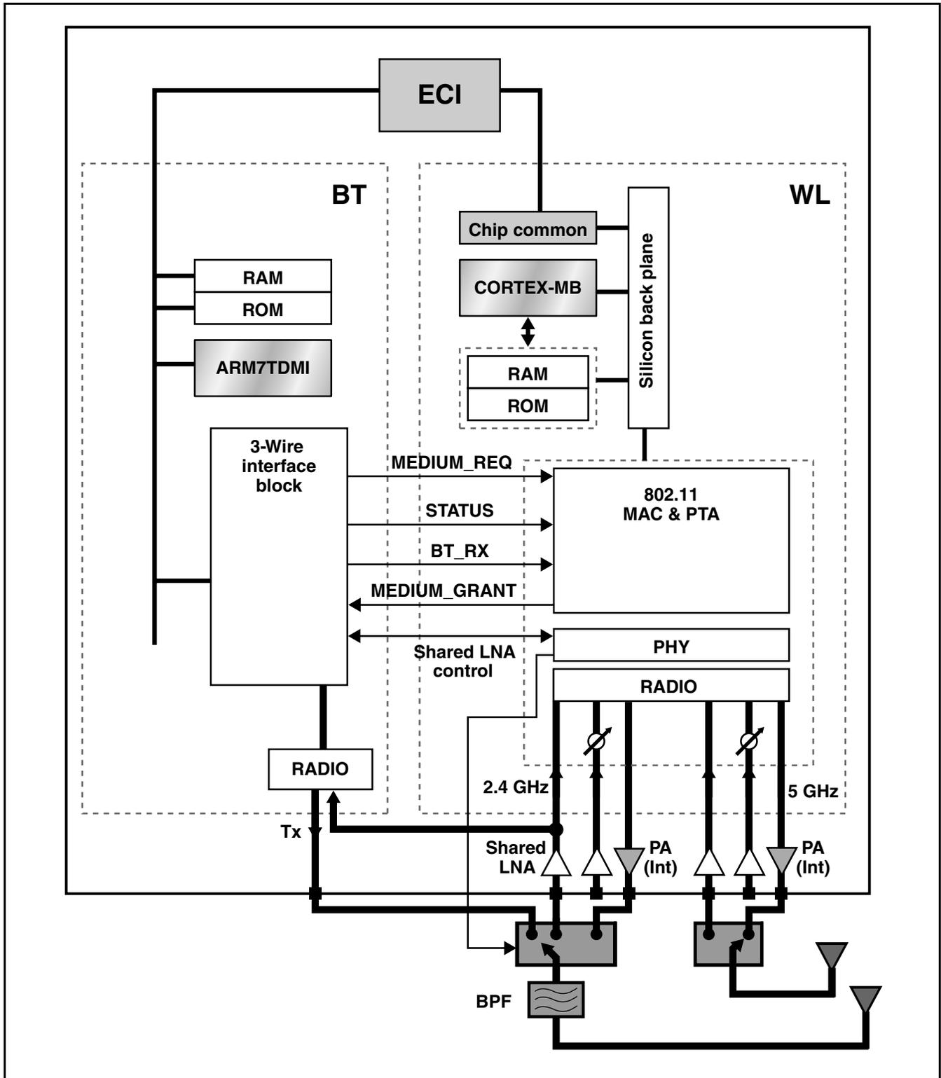
Figure 1: WLAN and Bluetooth Colocation Architecture
